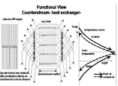
differences inside a room. The hr-efficiency becomes optimal, since the heat energy is transferred between equal-sized air volumes.
